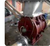
▶ ATEX version for a high explosion resistance and at the passage of flame
