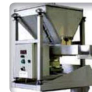
▶ Setting of the vibration amplitude (flow management)
