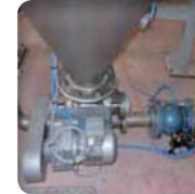
▶ Motorisations: direct by gear, coaxial variator with chain transmission or without motorisation (bare shaft)
