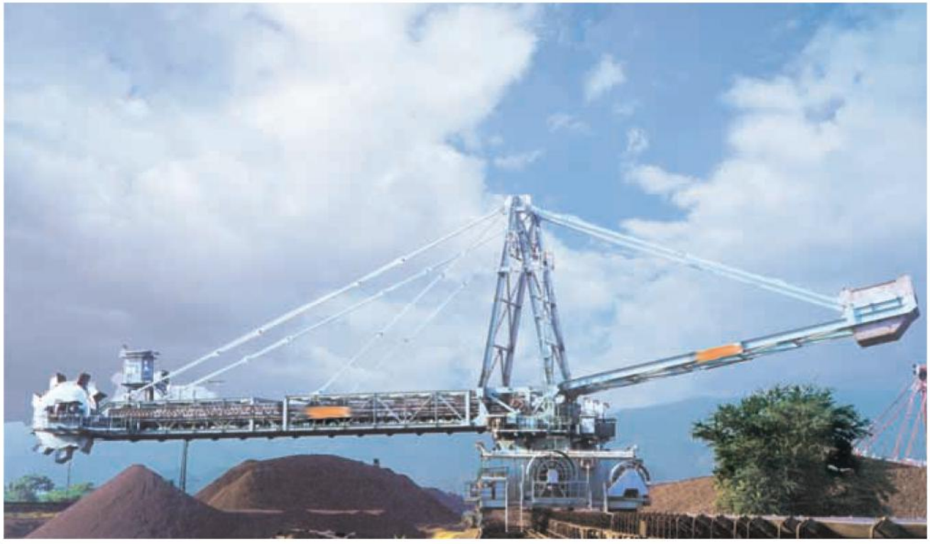
Wheel on Boom Reclaimer with 40 meters Boom Length handling Iron ore at 4000 MTPH capacity at izag Port Trust
